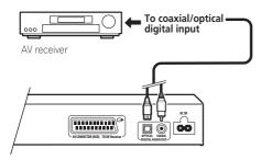
For an optical connection, use an optical cable (not supplied) to connect the OPTICAL **DIGITAL AUDIO OUT** jack to an optical input on your AV receiver.
